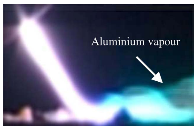
Fig. 5. Stable and constricted arc root on an aluminium anode precursor.
